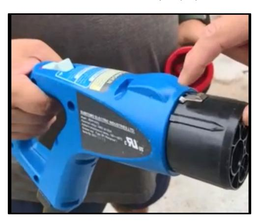
3. Carefully connect the CHAdeMO connector into the adapter or EV charging port. Ensure the connector is fully engaged. There will be an audible click, and no visible gaps.
